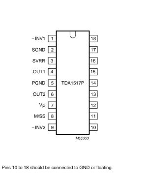
Fig.3 Pin configuration for SOT398-1.
